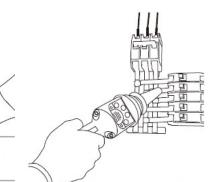
Voltage detection for a wall outlet
